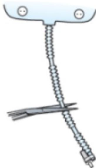
Figure 17. Cut the tubing
