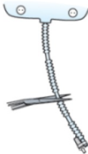
Figure 17. Cut the tubing
