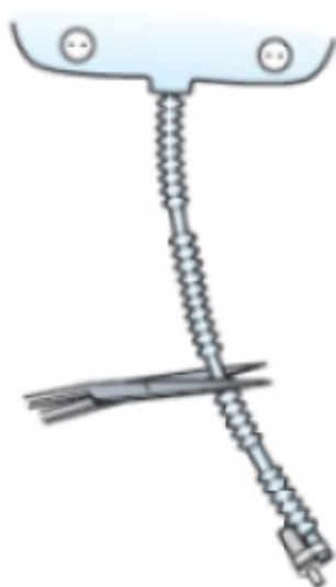
Figure 17. Cut the tubing
