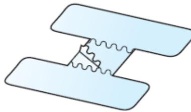
Figure 8. Removing backing from UC strip
