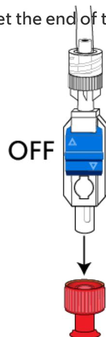
Figure 3. Flow switch in the “Off” position
