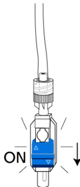
Figure 4. Flow switch in the “On” position
