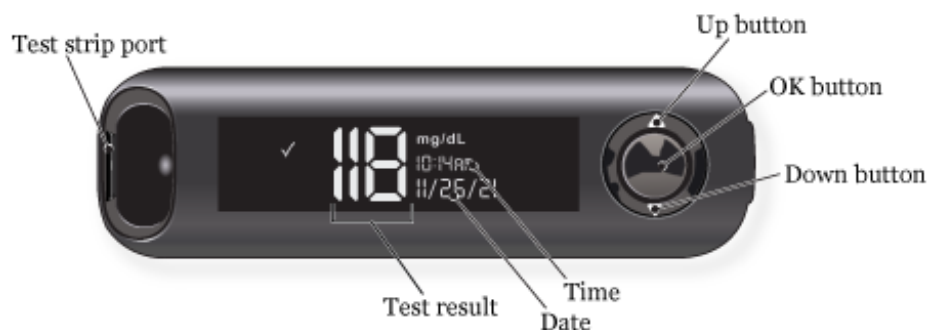
Figure 2. Contour Next One blood glucose meter
