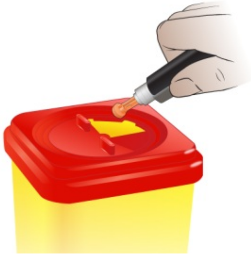
Figure 17. Eject the lancet into the sharps container
