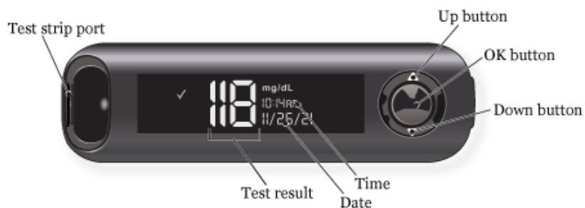
Figure 2. Contour Next One blood glucose meter
