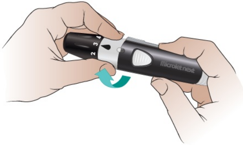
Figure 4. Twist the white band to the right
