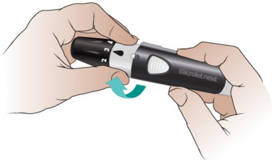
Figure 4. Twist the white band to the right
