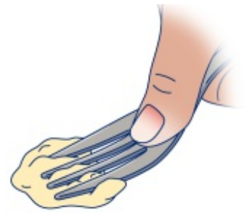
Figure 1. Fork or spoon pressure test
