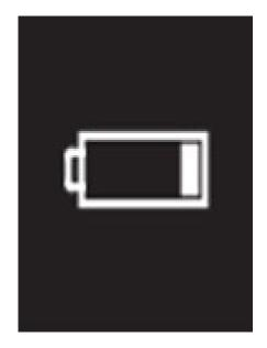
A low battery symbol will appear on the Nonin device when batteries need to be changed.
