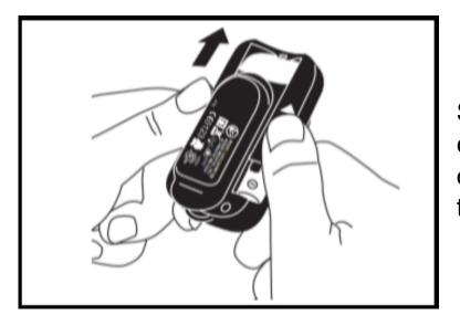
Slide off the back cover of the pulse oximeter and install two AAA batteries
