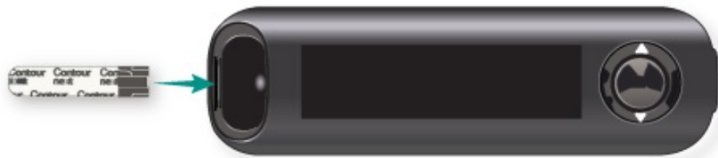
Figure 10. Put the test strip into the port
