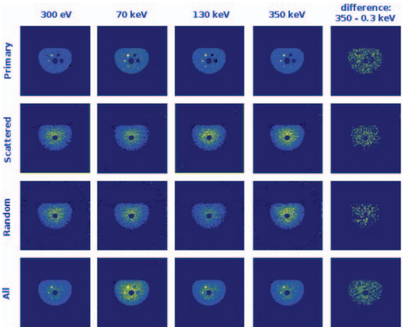
Fig. 3. Reconstructed images of the central slice of the NEMA IQ phantom. The images in each row correspond to a given cut, as indicated. The images in the final row are obtained by subtraction of the images for 0.3 keV cut from those for 350 keV cut. The images in each line are obtained from different types of coincidences as indicated. Each image is normalized to the most intensive pixel in it.
