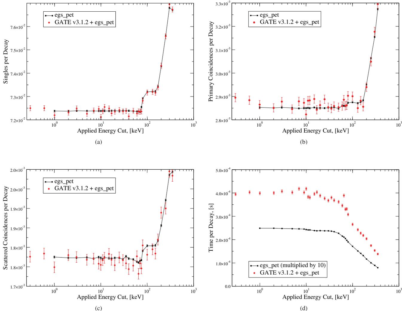
Fig. 1. Dependence of the number of singles (a), primary (b) and scattered (c) coincidences on the energy cut. (d) - Dependence of the simulation speed on the energy cut. In these simulations (scanner and a cubic water phantom with no voxels) egs\_pet is approximately 16 times faster than GATEv3.1.2+egs\_pet.
