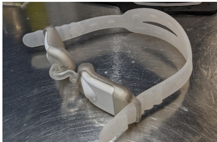
Fig. 1: Prototype incorporating silicon, Cerrobend, and 3D-printed parts.
