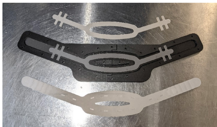
Fig. 2: Three-dimensional-printed mold for the strap.
